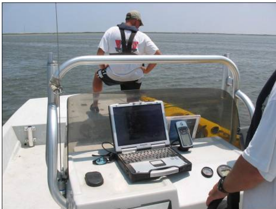
Figure 27. Field data entry setup in one of the Texas Parks and Wildlife Department boats. The link to the GPS receiver allows navigation directly to specific sites as displayed on the computer screen.
